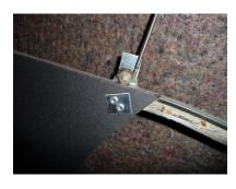
On the boot-lid Traction Avant, there are two pieces of carton that should go in the section between the rear doors and the rear window, on either side of the car. One is a smaller triangular piece. The other one has the shape of a large shell. Make sure to attach the small triangular pieces of carton as shown on the picture, using the screw of the hoop. The large pieces of carton
