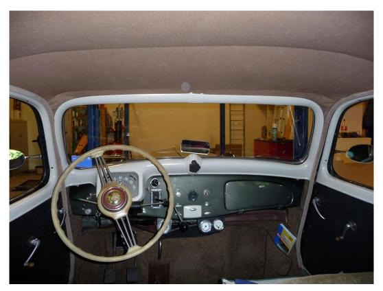
Finally, all the other fittings should be mounted, carefully cutting or punching neat holes in the lining cloth: the interior ceiling light (activated by the "P" switch on the dashboard, which stands for "Plafonnier"), the sun visors and —in the case of the 15/6- the hanging loops behind the rear doors.
