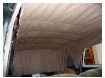
Carefully collect the complete lining with the hoops in place and climb into the back of the car, holding the cloth in the right position.
